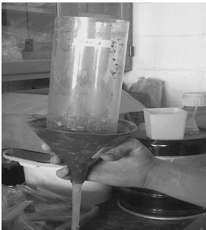
Fig. 6. Prototype of leaching columns designed for this study
