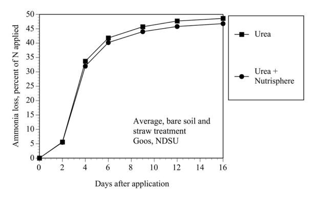
Procedure: Urea granules, and urea granules treated with Nutrisphere were obtained from the Simplot company. Bare soil, or bare soil with a ~50% cover with wheat straw was treated with fertilizer granules at a rate of 100 kg N ha<sup>-1</sup>. Ammonia volatilizing from the surface was trapped with phosphoric acid, and determined via the steam distillation method. This was a greenhouse study.
