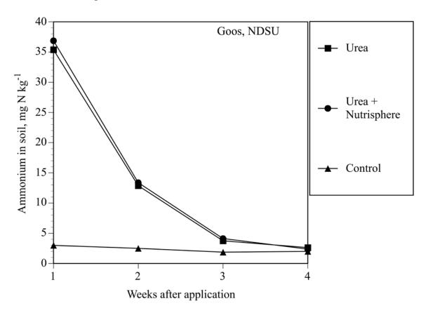
Procedure: Urea granules, or urea granules treated with Nutrisphere, were obtained from the Simplot company and used in a greenhouse study. Granules equivalent to 100 kg N ha<sup>-1</sup> were mixed with a sandy loam soil, and allowed to incubate for up to four weeks with minimal water movement. The initial N application to the soil was about 91 mg N kg<sup>-1</sup>. The soil was dried, sieved, and analyzed for KCl-extractable ammonium.
