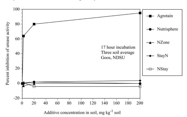
Study 9. Percent inhibition of urease given by different rates of various fertilizer additives.
